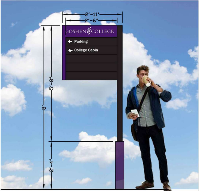
DIRECTIONAL SIGN 3 ELEVATION (NOT TO SCALE)
