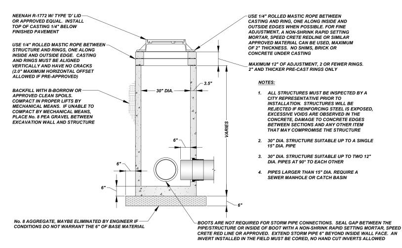
SEWER INLET (TYPE O) - FLAT CASTING
