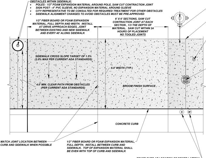
STAMP CURB AT LOCATION OF SEWER LATERAL AND WATER SERVICE, 2" MIN. TEXT SIZE
