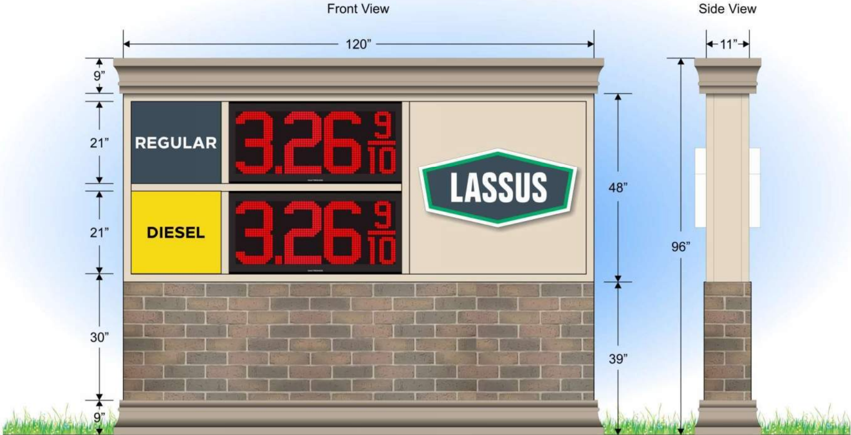
Double Face Monument Sign: Aluminum Cabinet with 2" Aluminum Divider Bars; Flat Faces Decorated with "Regular" & "Diesel" Graphics; (4) Daktronics Fuelight FL-5000 16" Fuel Digits; "Lassus" Flat Polycarbonate Face with Two Levels of Embossing; Decorative Aluminum Top Cap; Base to be Brick with Decorative Aluminum Bottom Cap.
