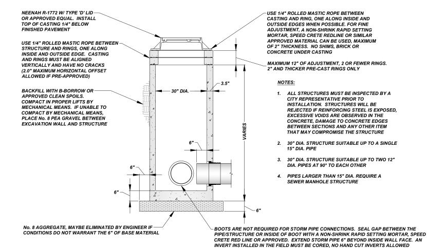
SEWER INLET (TYPE O) - FLAT CASTING
