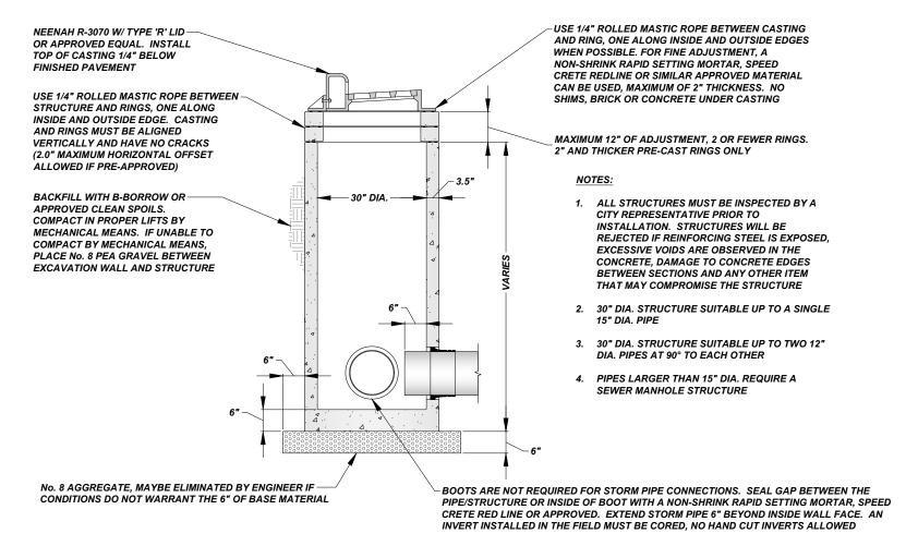
SEWER INLET (TYPE N) - CURB CASTING
