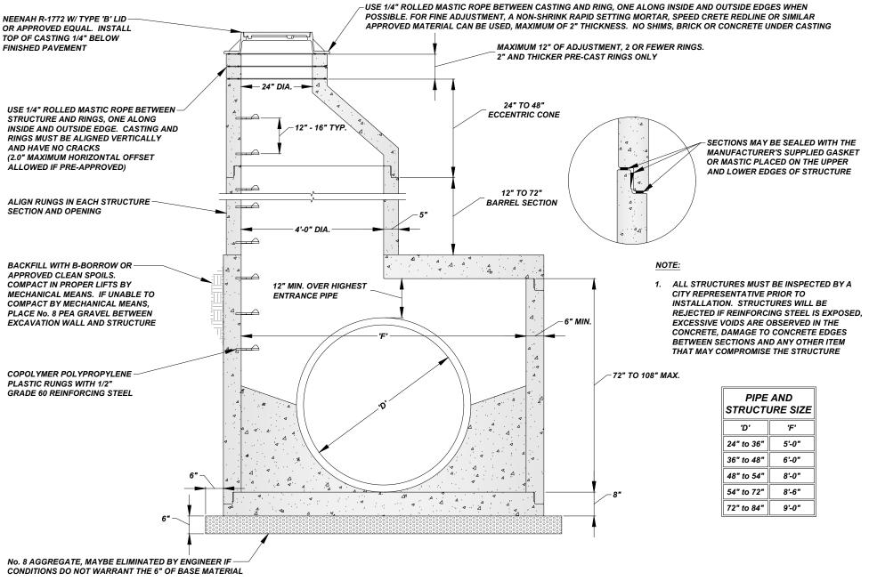
STEPPED SEWER MANHOLE (TYPE J) - CONE W/ MANHOLE CASTING
