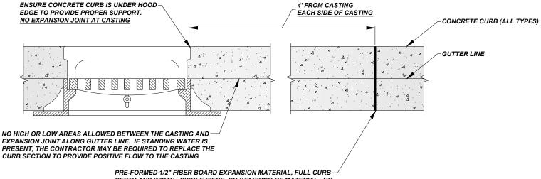
DEPTH AND WIDTH. SINGLE PIECE, NO STACKING OF MATERIAL. NO CONCRETE SHALL BE PLACED OVER THE JOINT. REPLACEMENT OF THE JOINT WILL BE REQUIRED IF EXPANSION MATERIAL IS NOT FULL DEPTH, FULL WIDTH AND/OR IS COVERED BY CONCRETE
