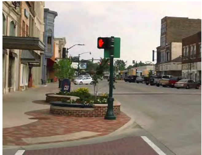
Figure 5. A bumpout in Elkhart (photo credit: Idris Busari, Youtube). Note: stamped asphalt crosswalks are uncomfortable for pedestrians using wheelchairs, using walkers, or pushing strollers.
