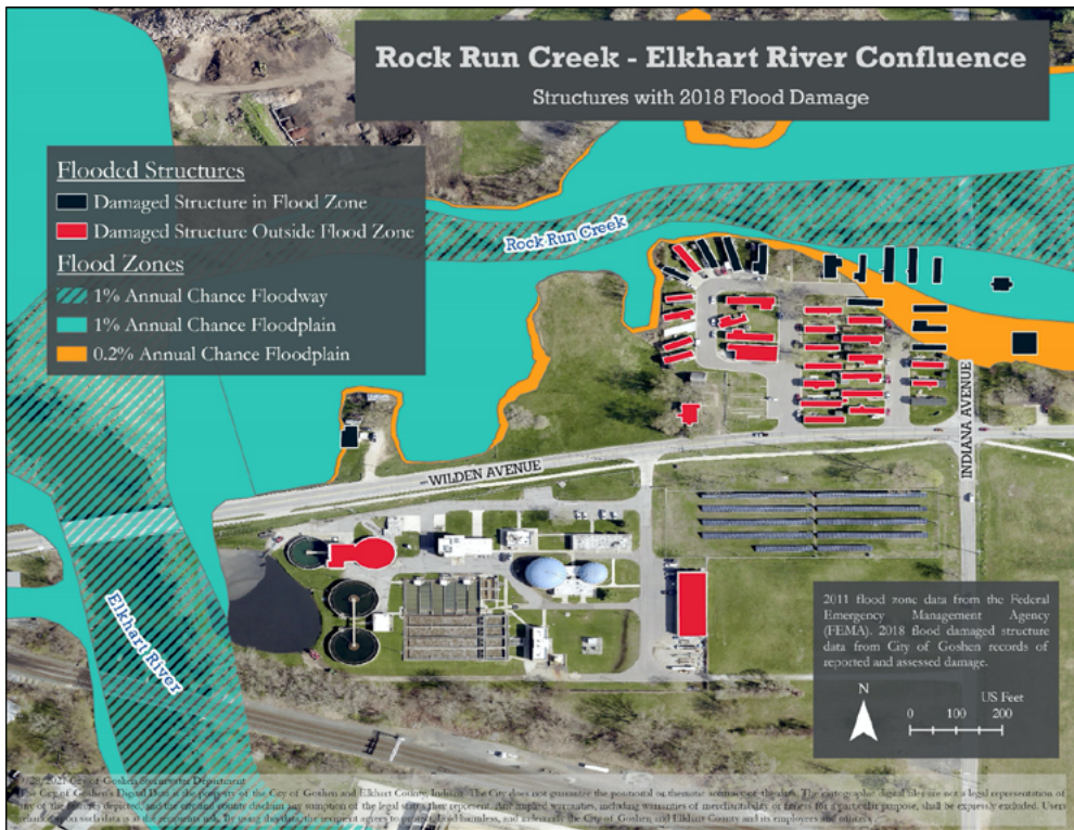
Figure 22: Structures with assessed 2018 flood damage along Wilden Avenue southeast of where Rock Run Creek empties into the Elkhart River.
