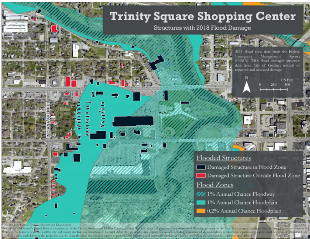
Figure 21: Structures with assessed 2018 flood damage in and surrounding Trinity Square Shopping Center.
