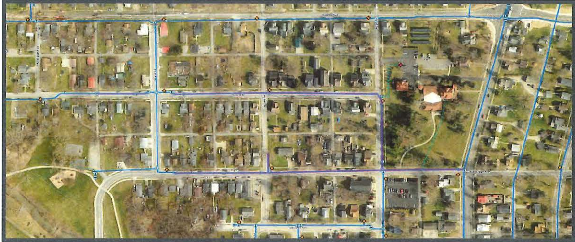
Figure 2: Water main replacements scope in Northside neighborhood
