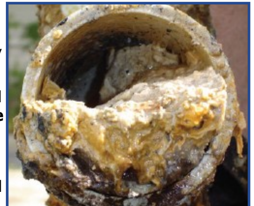
A clogged pipe caused by the dumping of FOG down the drain. Photo Credit: City of Elkhart
