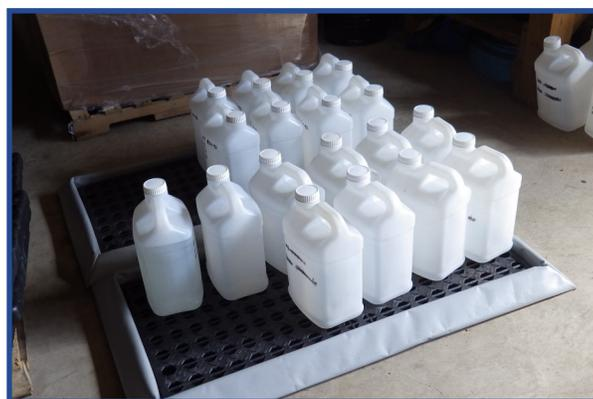
The secondary containment of materials helps to prevent accidental releases or spills of dangerous materials to our water, soil, and air. Secondary containment areas will vary in size and shape based upon the material being stored and the storage location. If you
