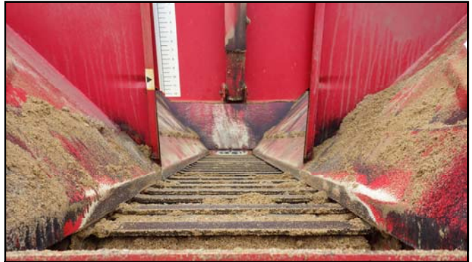
The conveyor belt of a hopper installed on the back of a Street Department dump truck.
