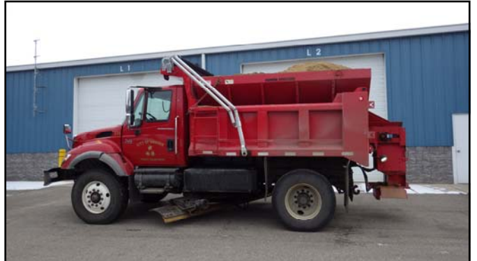
A Street Department dump truck outfitted to spread a mixture of sand and salt.
