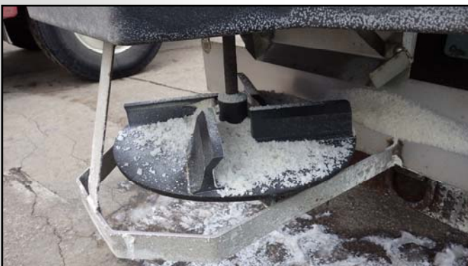
The spinner plate that helps spread salt and sand.
